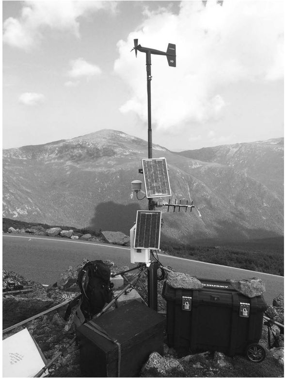
One of 18 weather stations that make up the Mount Washington Regional Mesonet.
