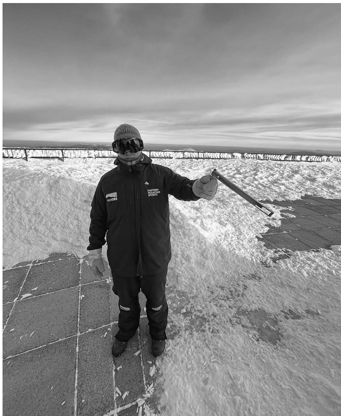
Former Weather Observer Hayden Pearson spins the sling psychrometer.
