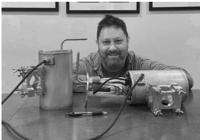
Mount Washington Observatory Director of Technology Keith Garrett is shown in North Conway, NH with the two pitot static tube anemometers custom-built for installation in May 2022 on Mount Everest.
