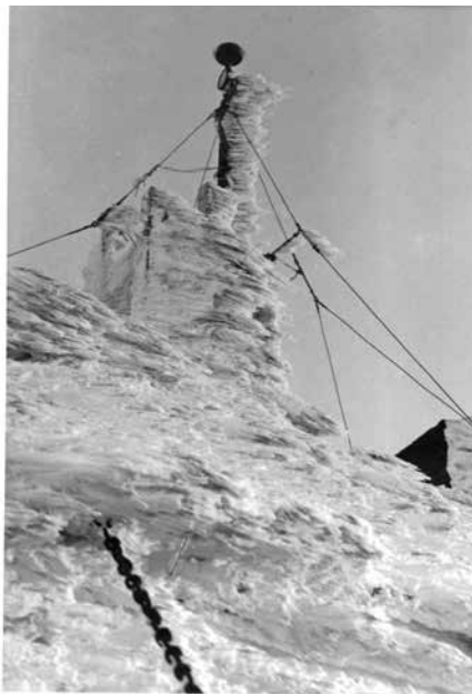
The “Heated No. 2” anemometer became the main wind sensor on the summit in 1933. It is most famous for recording The Big Wind of 231 mph on April 12, 1934, which still stands as the fastest surface wind speed ever observed by a human.
