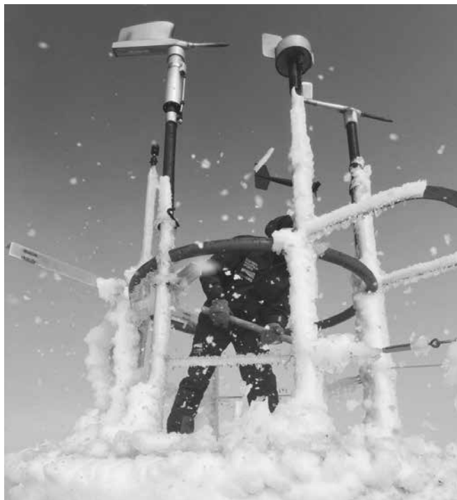
MWOBS/MWAC Intern Laura Wilson de-icing instruments at the top of the tower.
