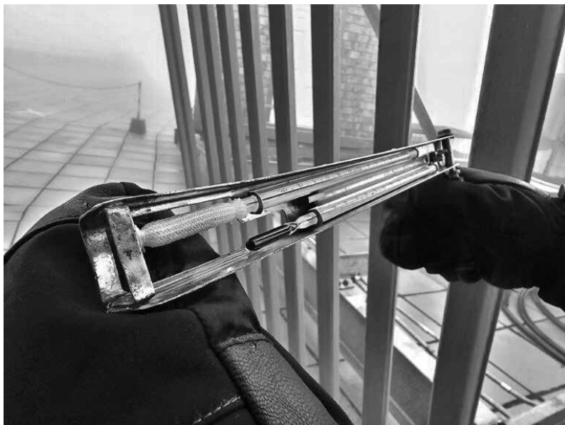
A Sling psychrometer: the wet bulb is wrapped in a cloth “sock” and stored in distilled water.
