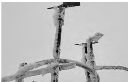
Below: Heavy icing of >9 inches per hour put the two pitot static tube anemometers, their heaters and the wind vane to the test. Photo by Adam Gill.
