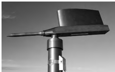
Left: The next-gen pitot static tube anemometer co-developed by General Electric aviation engineers, University of Massachusetts-Lowell engineering students, and MWO staff.
