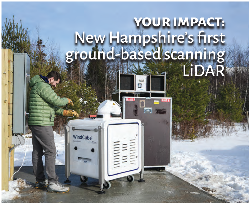
Director of Weather Operations Jay Broccolo installing the Vaisala WindCube 200S LiDAR in Bretton Woods in January 2026.
